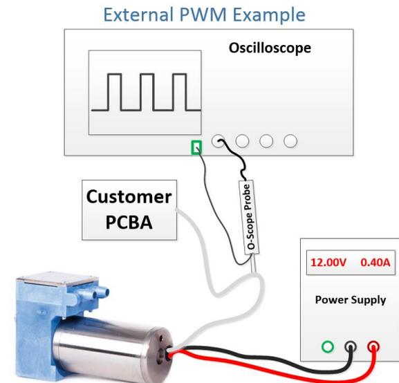
Most of Precision Fluidics diaphragm pumps with external PWM require an “open-drain” or “open-collector” circuit on the customer device PCBA to provide the PWM signal. The BLDC motors have an internal pull-up resistor so the open-drain or open-collector circuits will actively bring this voltage to ground for the low part of the PWM signal. The illustrations below show the generic recommended circuits.
