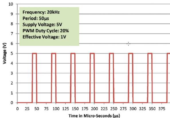
*Example of a 20% Duty Cycle PWM Signal*
