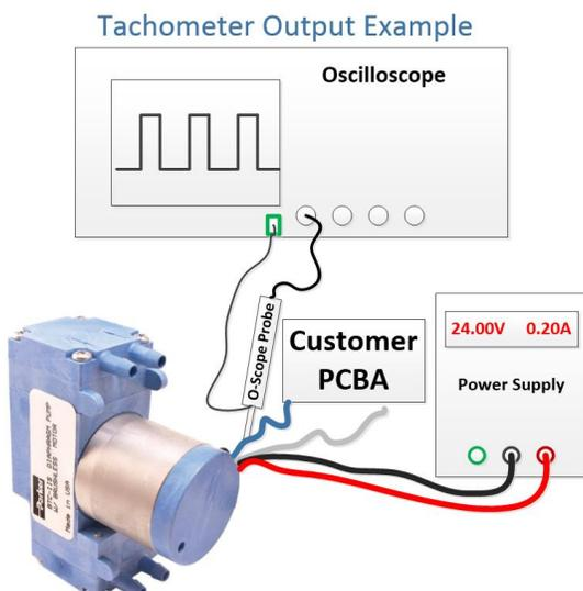
Example of Tachometer Output Signal
