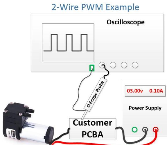
For brush motors, it is the most common method for control, and very effective. Likewise with BLDC motors, it is effective; however, it does present some limitations. Precision Fluidics BLDC motors have an internal controller that must maintain a minimum voltage to operate properly. When applying a PWM cycle to the input voltage it is also
