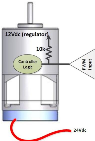
24 Vdc High-Torque BLDC Internal Circuit
