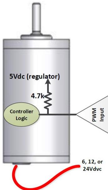
6, 12, or 24 Vdc Premium BLDC Internal Circuit
