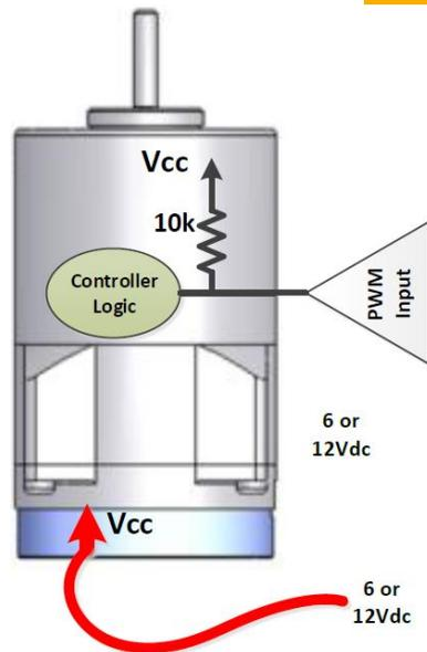
6 or 12 Vdc High-Torque BLDC Internal Circuit
