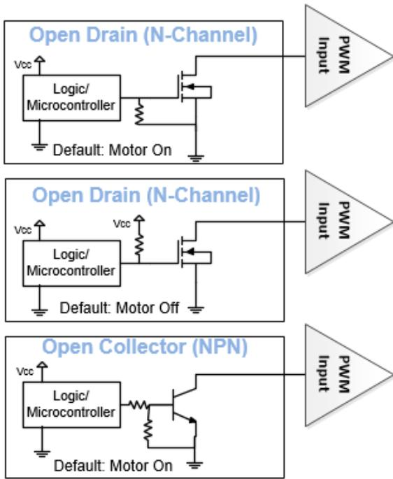
Open-Drain/Open-Collector Circuit Examples
