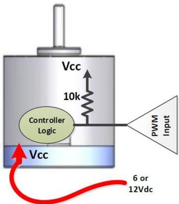
6 or 12 Vdc Standard BLDC Internal Circuit
