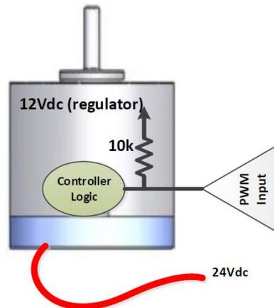
24 Vdc Standard BLDC Internal Circuit
