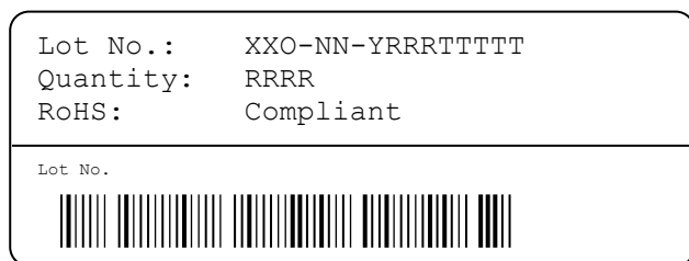
Figure 20: First label on reel: XX = Sensor Type (25 for SHT25), O = Output mode (D = Digital), NN = product revision no., Y = last digit of year, RRR = number of sensors on reel divided by 10 (200 for 2000 units), TTTT = Traceability Code.
