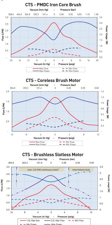
The above graphs represent an example of performance for the pump series handling air at 800 feet (244 m) above sea level at 75°F (24°C). Performance will vary depending on barometric pressure and media temperature. A variety of configurations can be accommodated to meet application requirements. Curves are representative of standard pump configurations. Pump configurations could be customized for higher or lower flows depending on specific customer requirements.
