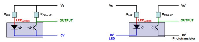
Note: The 4-wire version provides galvanic isolation between input (IR-LED) and output (Phototransistor).
