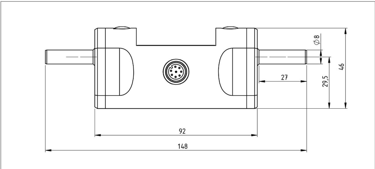
Figure 1: Dimensions SONOFLOW® IL.52/3 V2.0 – Side view
