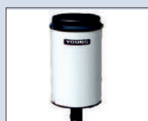
Young 52202/03 Tipping Bucket Rain Gauge This rain gauge comes with a catchment area of 200 cm 2 and a resolution of 0.1mm. Can be de- ployed on flat surfaces or mounted to a pole. D=180mm, H=300mm
