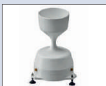
ARG314 Tipping Bucket Rain Gauge Resolution 0.1/0.2/0.5mm (options) Aerodynamic rain gauge made of UV resistant injection moulded plastic with self-emptying tipping bucket. (datasheet seperately available)
