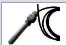
DKRF370 - Humidity/temperature probe for compressed air up to 100 bar, G3/8" thread, Operating conditions: -20...+80°C. Dimensions: 100mm x 13mm
