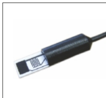
SHS-325 - Detects incipient bedewing. Signal "1" if condensation occurs, "0" if not. Operating range: 0...50°C Dimensions: 60 x 10mm
