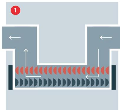
SONOFLOW flow meters use the transit-time ultrasound method to accurately determine the flow rate. The sensor measures the time of flight of the ultrasonic wave with and against the streaming liquid.
