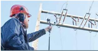
→ Detect partial discharges at an early stage and increase operational reliability
