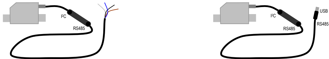
Figure 1: SCC1 cable connected to a sensor with pigtail cable (left) and with USB plug (right). Communication interfaces shown in small print.
