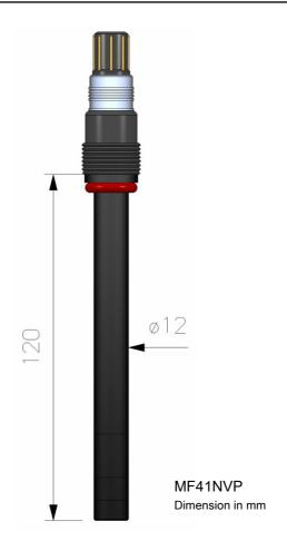
The amperometric oxygen probe is ideal for direct control of dissolved oxygen in water, e.g. drainwater, surface water, fish farming or laboratory and engineering plants. The oxygen probe MF41N features high long-term stability, low maintenance and identical dimensions to pH-electrodes.
