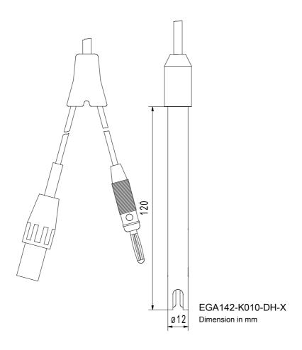
This low maintenance pH combination electrode with gel electrolyte, rugged plastic shaft and built-in temperature probe is used especially in connection with laboratory and field instrumentation. The sensor features application in water technology, sewage treatment, environmental analytics and aquaristics. The incorporated temperature probe allows simultaneous measurement of pH and temperature especially for automatically temperature compensated pH measurements.
