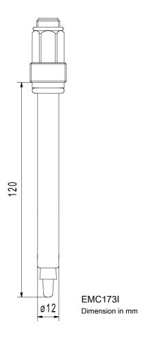
This Redox/ORP combination electrode with gel electrolyte and large-sized ring shaped fixed glass sleeve junction features application under industrial conditions in water technology, sewage treatment, electroplating and process chemistry. The platinum disc increases mechanical stability and decreases dependence on flow.
