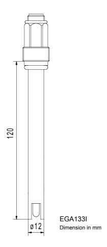
This low maintenance pH combination electrode with gel electrolyte and plastic body is recommended for general application in aquariums, water and waste water technology as well as in water treatment for swimming pools.
