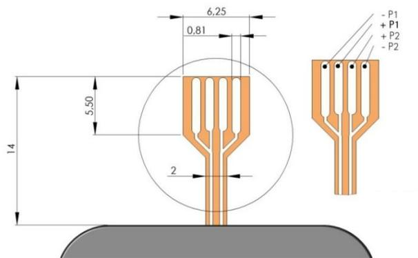
Figure 16 Schematic of the FCC connector of the mp6 micropump; all dimensions in [mm]
