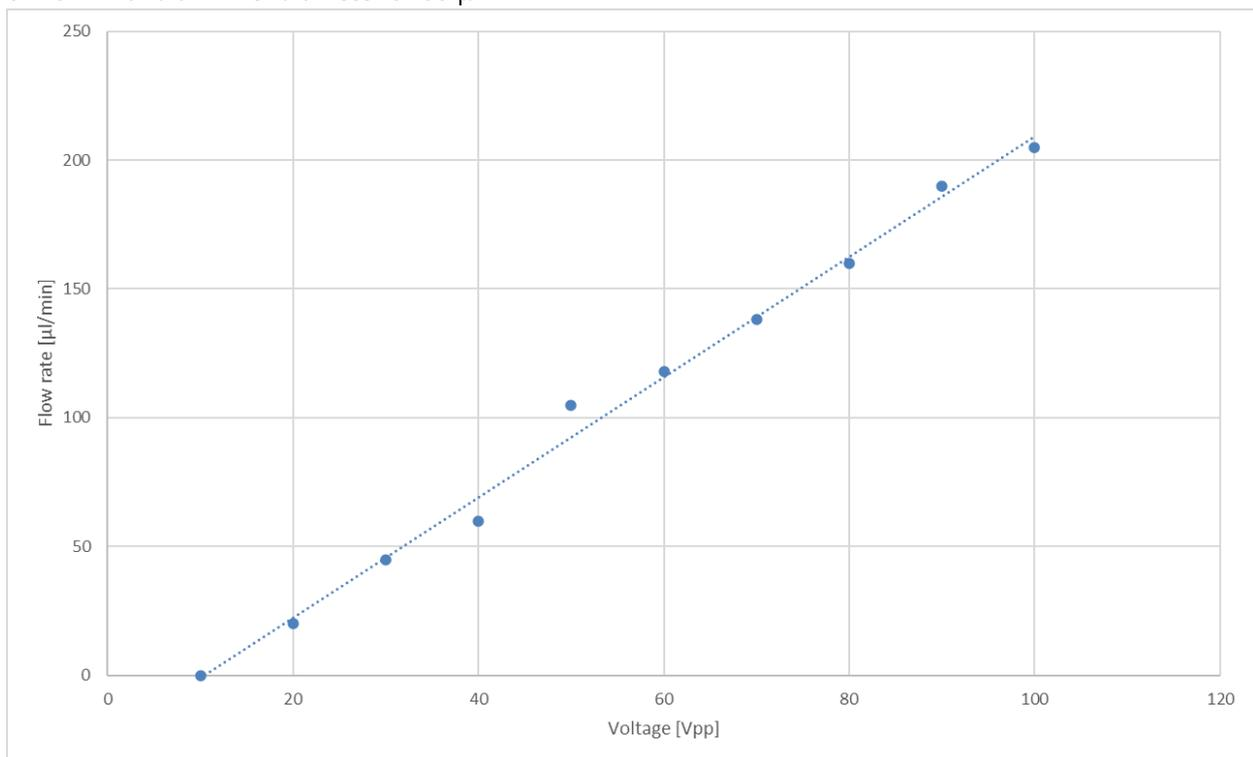
Figure 14 Flow restriction utilizing capillary l = 70 mm and ID = 65 µm with mp-Highdriver at 50 Hz pump frequency
