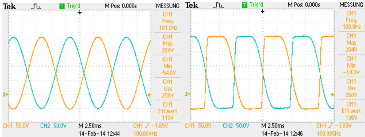
Figure 15 Scopeshots of a mp6 micropump at 250Vpp; 100 Hz; sine signal (left); SRS signal (right) / Voltage at piezo actuator 1  $\triangleq$  CH1 & piezo actuator 2  $\triangleq$  CH2
