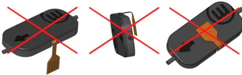
Figure 10 Important notes about the proper use of the flexible connector
