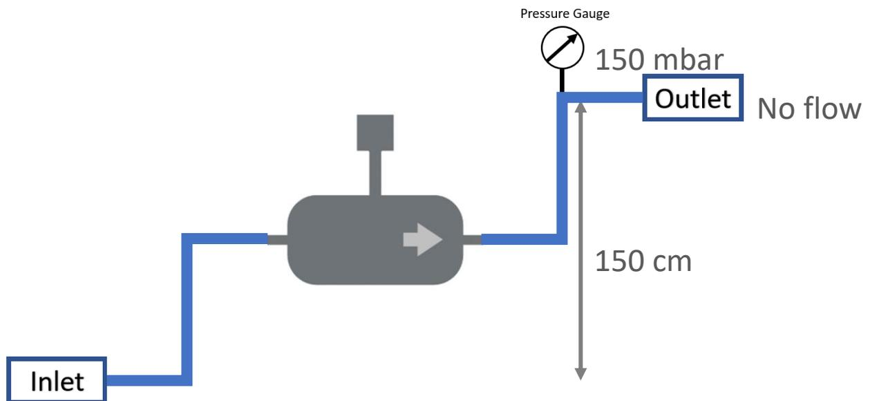
Figure 3 Example increased pressure due to height difference in the system
