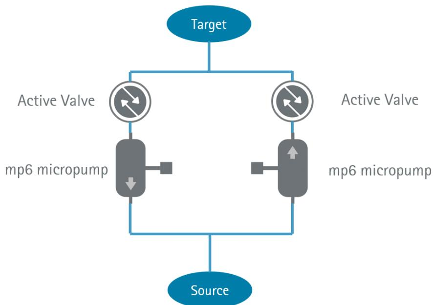
Figure 10 Block diagram for using two micropumps in opposite direction and two 2/2-way valves
