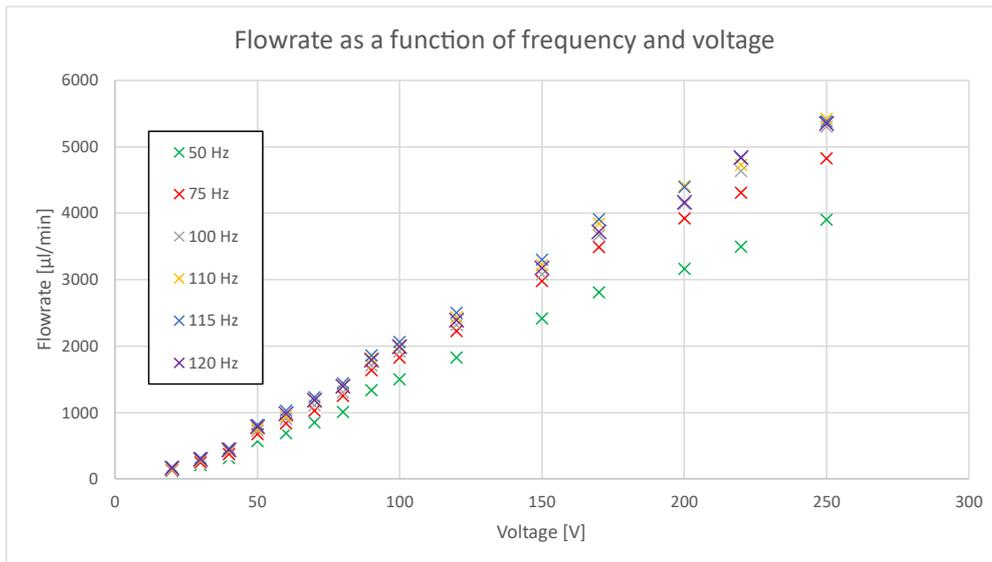
Figure 13 Example mp6 run by mp-Highdriver pumping water (low frequencies)
