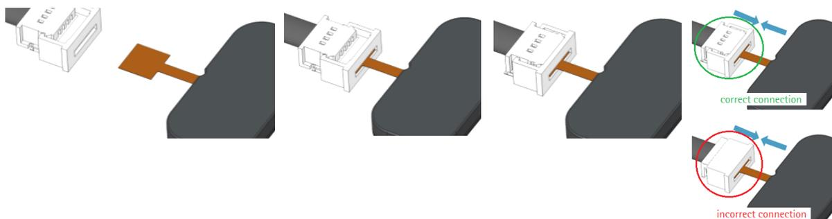
Figure 9 How to connect the mp6 micropump to the Molex connector
