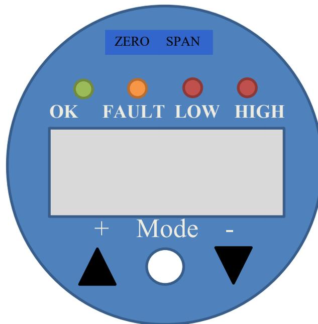
The blind Sensotox 2 have a small seven segments display with three mechanical keys: [+], [MODE] and [-] on the main board. The data to be displayed will have up to 4 digits, displayed sequentially. The first digit is distinguished because the off time is longer than the rest. For example, for to show data 1234 would be:
