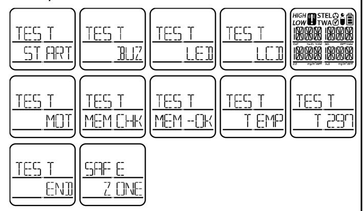
Press and hold the button for 3 seconds. The device will start the self-test checking buzzer, LED, LCD, Motor, Memory, and Temperature.
