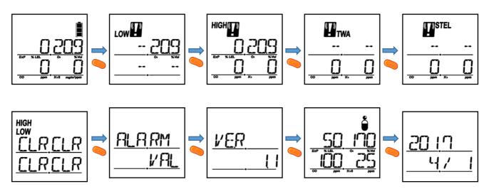
The displays in ten different modes as above are shown in the measuring mode every time when you press the KEY button( ).
