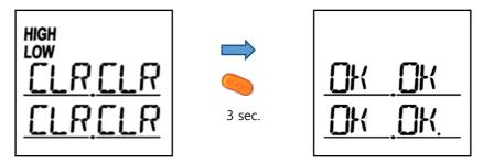
You can see the minimum and maximum values for the concentration levels detected by the device as well as the high TWA and STEL value on the display, and the values can be initialized. Press KEY button ( ) for three seconds on the CLR(Clear) mode on the LCD monitor, and the OK will appear on the LCD monitor to notify the completion of the initialization.
