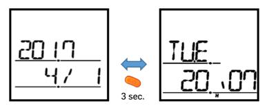
Press the button ( ) under the (YY/MM/DD) mode for 3 seconds and the day/time mode will appear. Press the button ( ) again for 3 seconds under the (D/T) mode and it will go back to previous mode.
