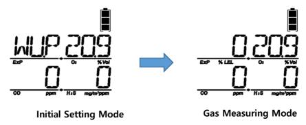
Once activated, the device will enter the warm up stage to stablize sensors. The warm up process is completed, the device is ready to detect gases.
