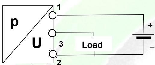
$$RI \geq 5 \text{ k}\Omega \quad 14 \dots 30 \text{ V DC}$$
