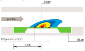
Figure 2: Cross-section view of the gas channel.
