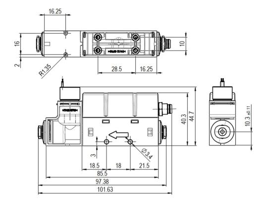
Figure 5: Physical dimensions and mounting information for SFC6000D with push-in fittings. All units are in [mm].
