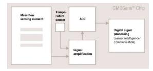
Figure 1: CMOSens® flow sensor diagram.
